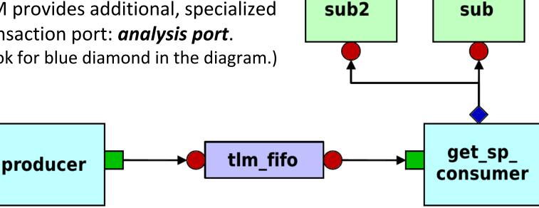
tlm analysis port has just one interface method write (void function) and can be connected to analysis exports of multiple data-collecting components (scoreboards, coverage collectors, etc.)
