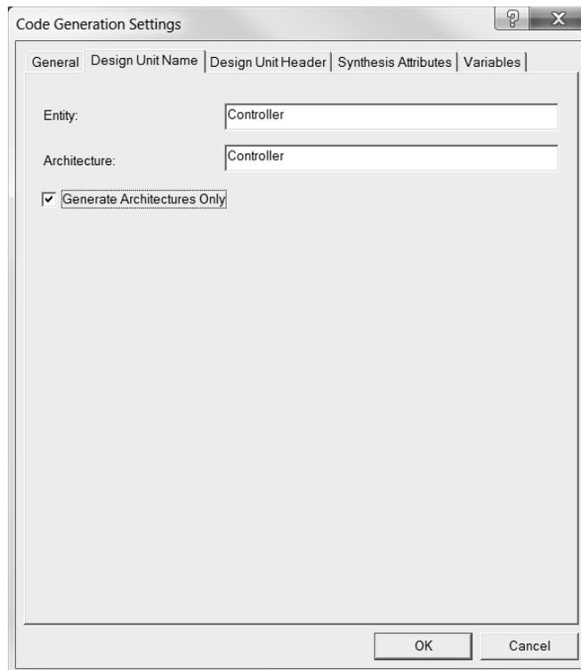
Figure 17: FSM Code Generation Settings - Design Unit Name
