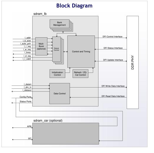
memory timing parameters and configuration settings. This ensures compatibility with all LPDDR3 SDRAM configurations.
