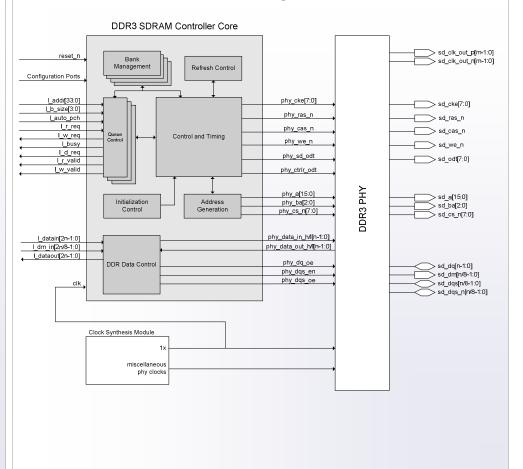
memory timing parameters and configuration settings. This ensures compatibility with all DDR3 SDRAM configurations. The core also supports of ODT, dynamic ODT, 2T timing and write leveling calibration.
